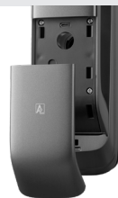
Emergency Power Mechanical Key
